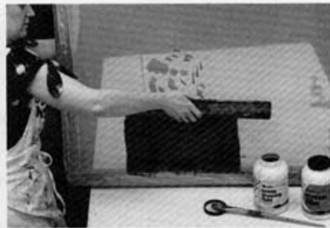
After drawing fluid image has dried, a thin layer of screen filler is scoop coated onto mesh.
