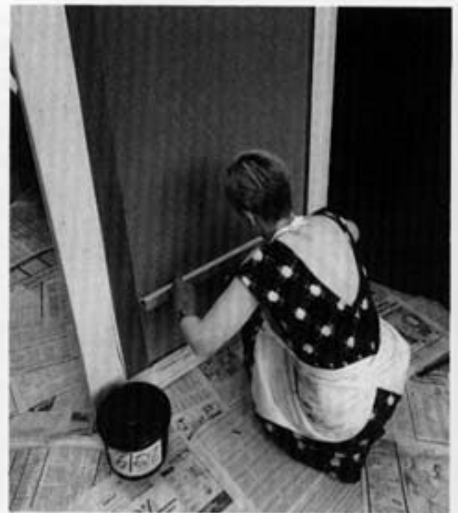
Using a scoop coater, firm pressure is required to ensure a thin even coating of photo emulsion.
