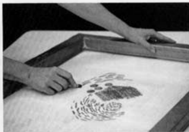
A flat surface is recommended for applying wax crayon to screen mesh.
